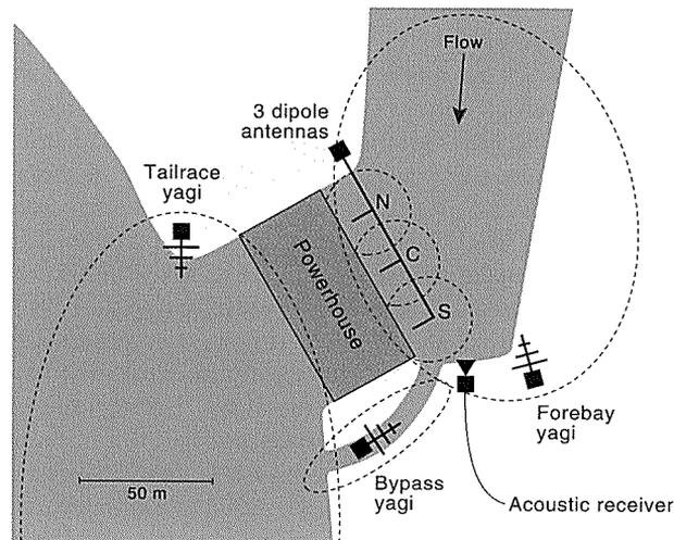
Figure 2. Plan view of Cabot Station and locations of datalogging radio telemetry receivers and antennas. Forebay dipole antennas (N, C, and S denote North, Center, and South, respectively) were interfaced to a single receiver. A datalogging acoustic receiver was installed at the downstream-most end of the forebay.
