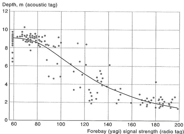
Figure 3. Relationship between radio-tag depth (as measured from acoustic tag) and signal strength from the forebay yagi antenna. Nonlinear regression (line) was used to infer depths of eels carrying only radio tags.
