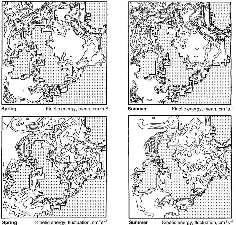
Fig. 2A. Seasonal means of the energy of the mean flow and of flow-fluctuations within the season.
