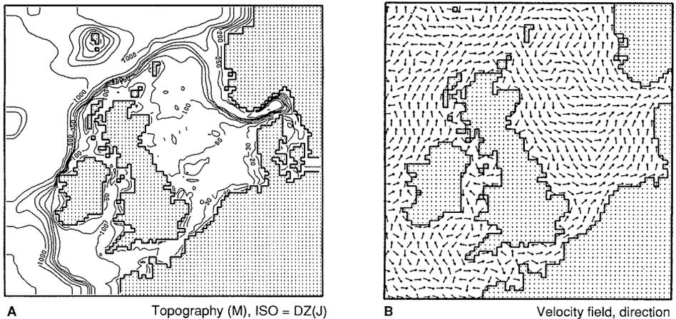
Fig. 3. A, topography of the North Sea and adjacent regions defined on discrete model grid (raster). B, mean direction of the flow within the North Sea (unit vectors).
