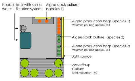
Fig. 2.7. A schematic overview of the live feed section used for producing algae and copepods for use in experiments with feeding larvae.
