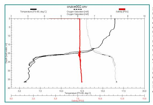
Fig. 6.5. An example of the data obtained with CTD probe send the down with the release container. The release in this particular example was performed at 22 meter depth. This corresponds to а temperature of 12 deg., salinity at 7.5 ‰ and a oxygen level at 8.0 ml/l. The red curve is oxygen in ml/l, the dark gray is temperature in degrees Celsius, the green is salinity in ‰, and the light gray is time used during the release.
