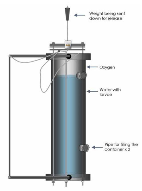
**Fig. 6.1.** The Release Beast built for the release of cod larvae. The blue depicts water with larvae. The cavity above the water level is filled with oxygen. For release, the weight is sent down along the main carrying wire hitting the release mechanism. The main body and the container then drops, pulling up the left-pointing arms and opening the butterfly valves that sealed the container during transport.
