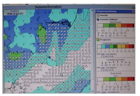
**Fig. 6.3.** A screen-shot of the actual currents and wind speeds prior to a release cruise. The currents shown with the white arrows indicate the currents found at 20 m depth. The data is available at <u>www.frv.dk</u>
