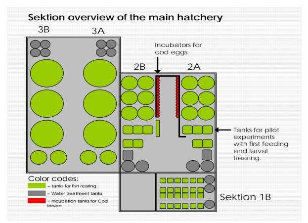
**Fig. 2.5.** This figure is a schematic overview of the main hatchery. The numbers 1A to 3B refers to Sections. Section 2 was used for the incubation of cod larvae and pilot investigations on first feeding in 2005-2007.
