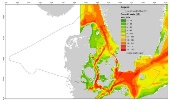
Figure 4. Example of BIAS Soundscape. Median map for the 125 Hz 1/3-octave frequency band and 10th percentile, for the full water column in January 2014. Sound levels in dB re 1µPa.
