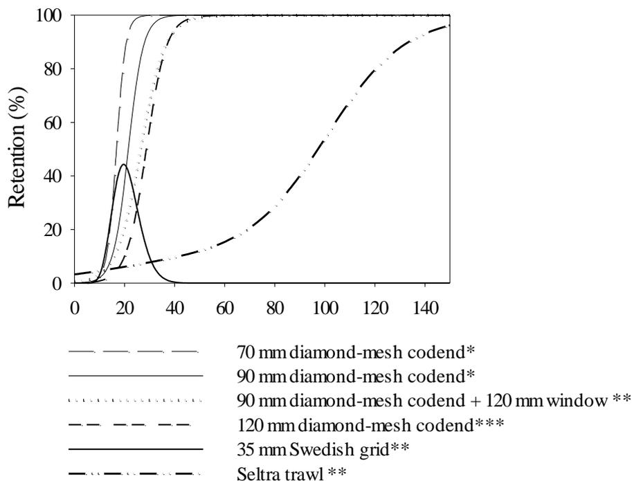
Figure 3. Cod selection curves for different gears according to minimum allowed mesh/bar size specified in previous (\*) or current (\*\*) legislation for the Kattegat and Skagerrak and in current legislation for the North Sea (\*\*\*). Figure from Madsen and Valentinsson (2010).
