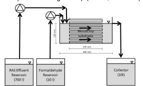
b) Recirculated set-up (Trial 2, side view)
