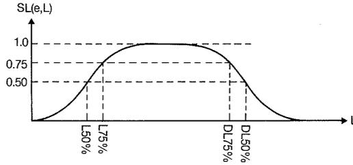
Fig. 1. Gear selection curve.
