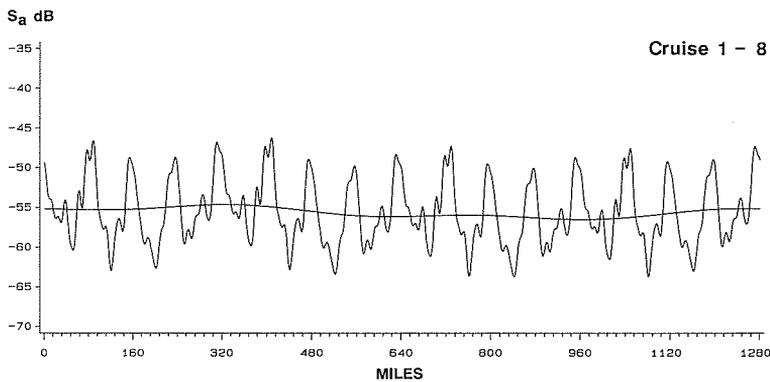
Fig. 4.  $S_a$  as composed of a trend and a periodic component. Trend = (mean +) oscillations with frequencies 1, 2 and 3. Periodic component = sum of oscillations with frequencies  $4 \cdot N$ ,  $N = 1, \dots, 26$ . Period = 320 miles.
