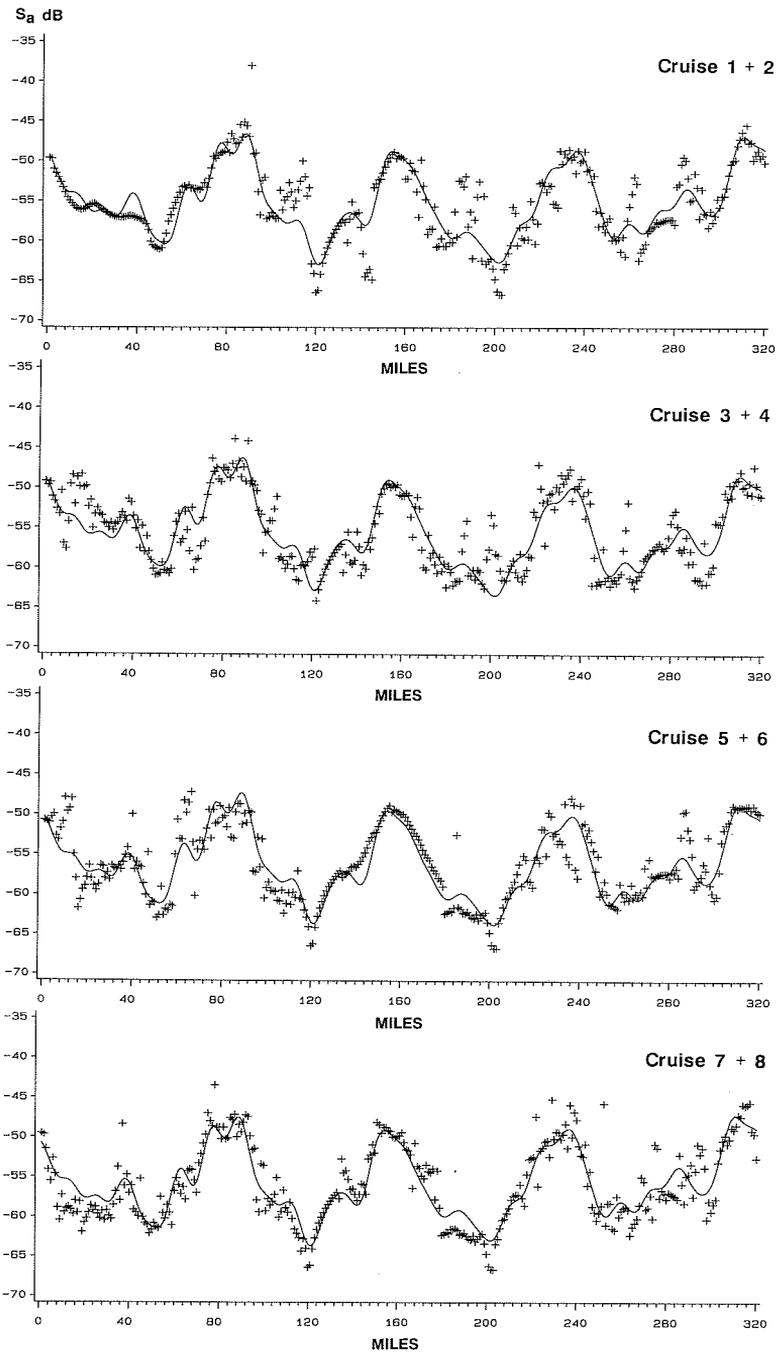
Fig. 3.  $S_a$  as function of mileage. + = observations — = sum of mean and oscillations with frequencies 1, 2, 3, 4, 8, 12, 16, 20, 24, 28, 32, 36, 40, 44, 48, 52, 56, 60, 64, 68, 72, 76, 80, 84, 88, 92, 96, 100, 104.
