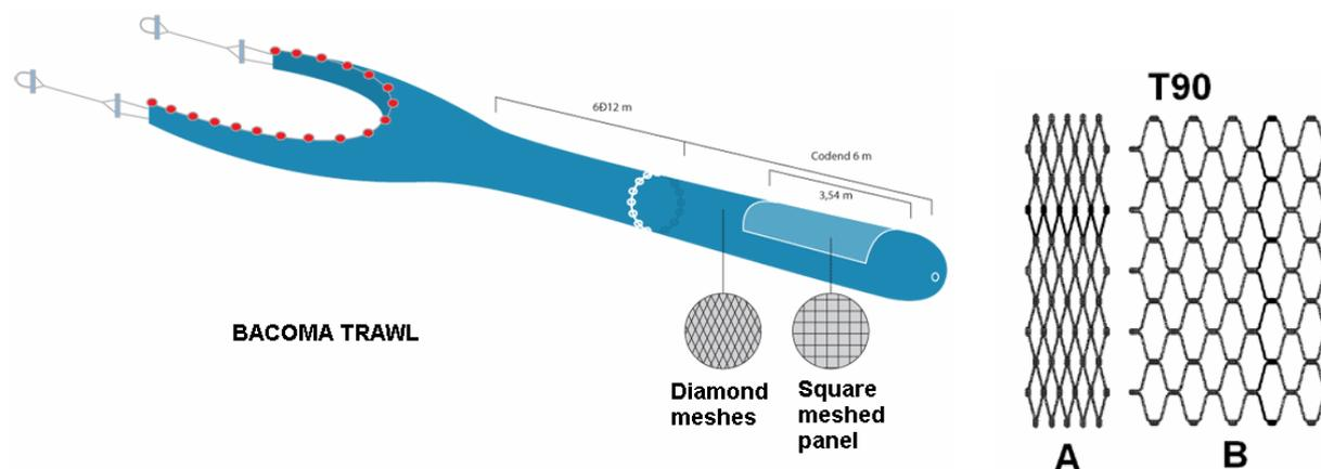
Figure F.4.4.1. Idealized picture of the Bacoma trawl and T90 Codend. (Modified from Swedish Board of Fisheries website: <http://www.fiskeriverket.se/laborationer/havsfiske/publikationer.htm>)
