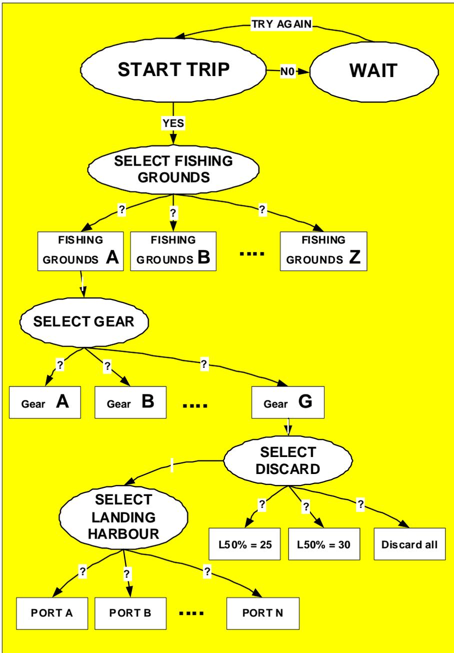
Figure B.2.5.1. shows an example of a decision tree for the trip related behaviour. In this case the decisions also include the selection of landing harbour. Making the choice of landing harbour a trip specific choice depends on the actual case. If vessels always land in the same harbour, say the home port, then there is obviously no reason to consider the landing port as a choice.
