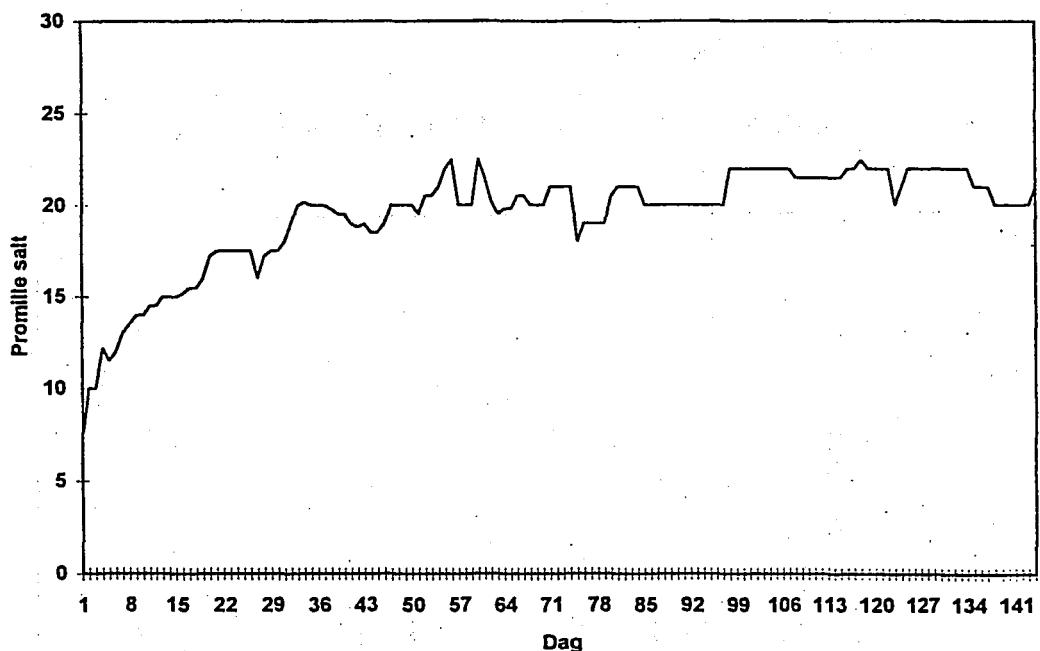
The great number of fluctuations in fig 1 were caused by periodic supplies of large quantities of 14‰ Østersø water pumped up from a depth of about 70 m and landed by "Jens Væver". After each supply the readjustment of the salinity would go on for some time.
