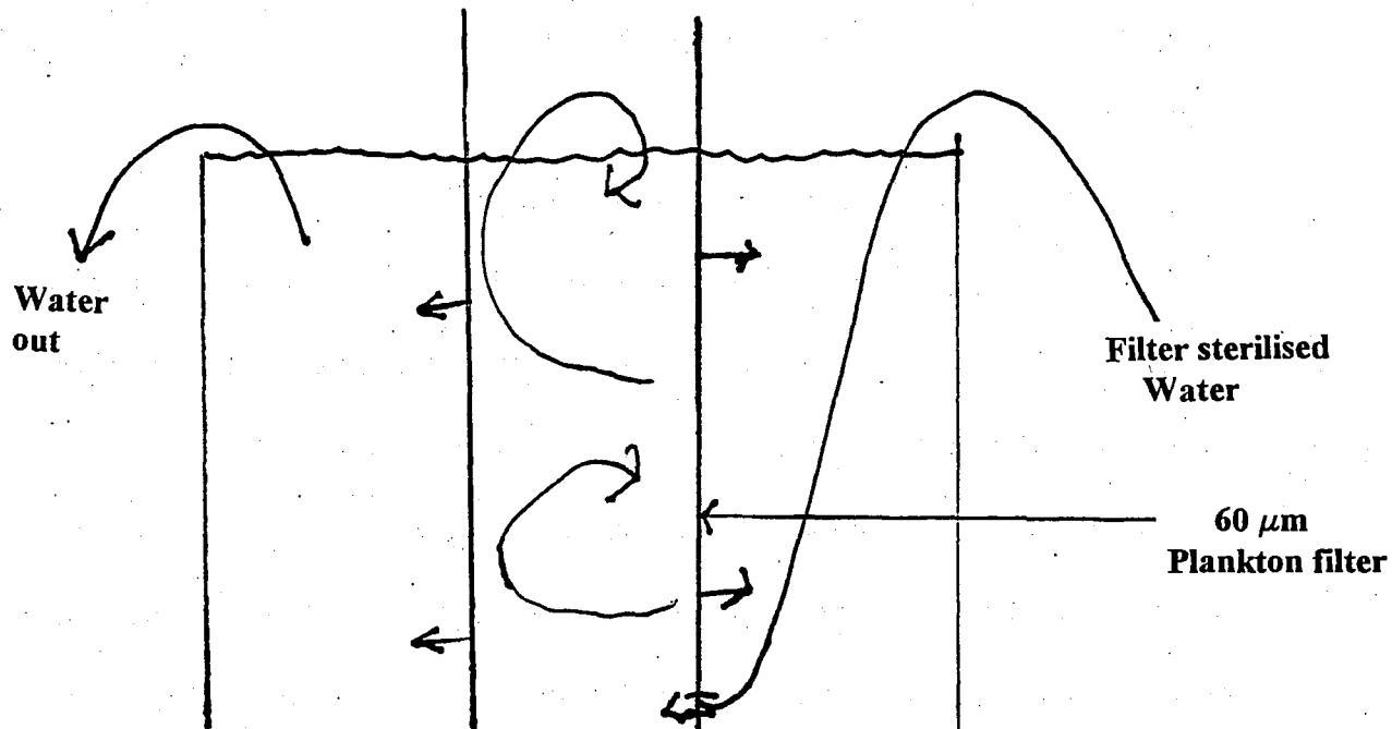
The advantage of this filter is the presence of a very large filter surface. Besides, the continuous addition of filter-sterilized water creates a rotation of the filtrate which leads to an effective straining off of secondary material. The water in the tank in which the filter is immersed creates a counterpressure that brings about a careful filtration of the rotifers.
