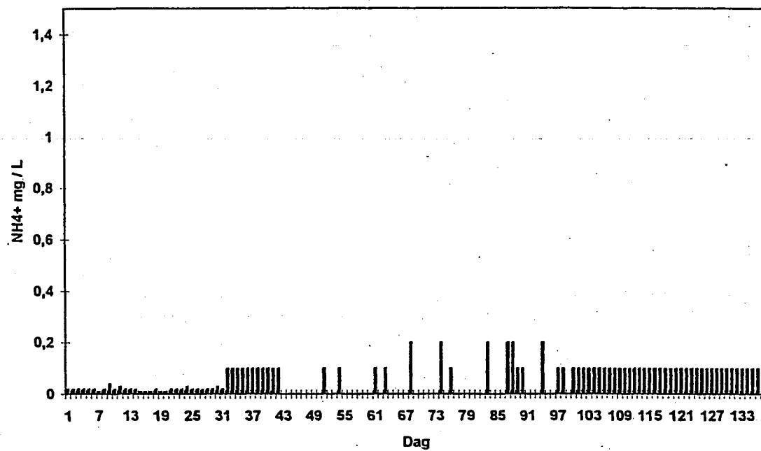
It appears that the concentration level is considerably lower than in the previous year - 0.2 mg/l with an average below 0.1 mg/l. This is partly due to an enlargement of the bio-screen capacity and partly to the fact that the filters had been inoculated with Nitrosomas and Nitrobacter bacteria the main capacity of which being the ability to convert ammonia and nitrite into nitrate.
