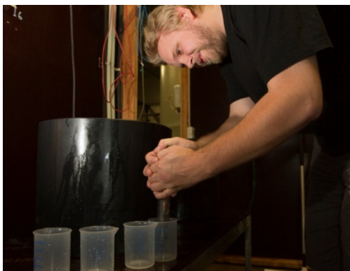
Figure 4.5.1. Monitoring procedure for accurate estimation of number of eggs incubated and fertilisation rate and subsequent mortality during incubation.
