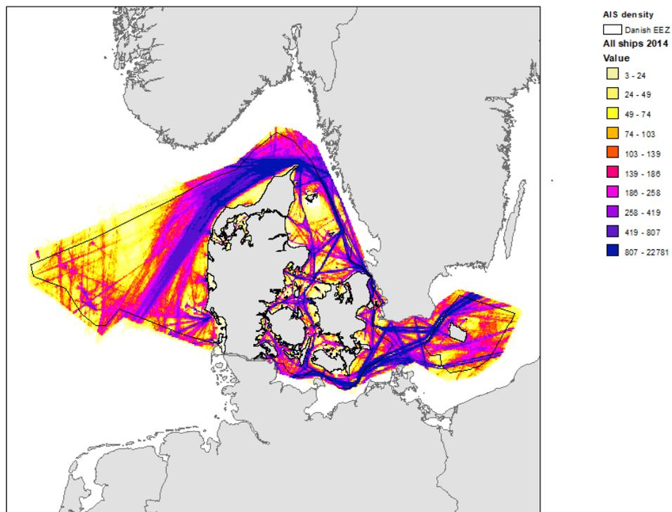
Figure 22.1. Map of the marine traffic intensity given as number of ship tracks per cell per year.
