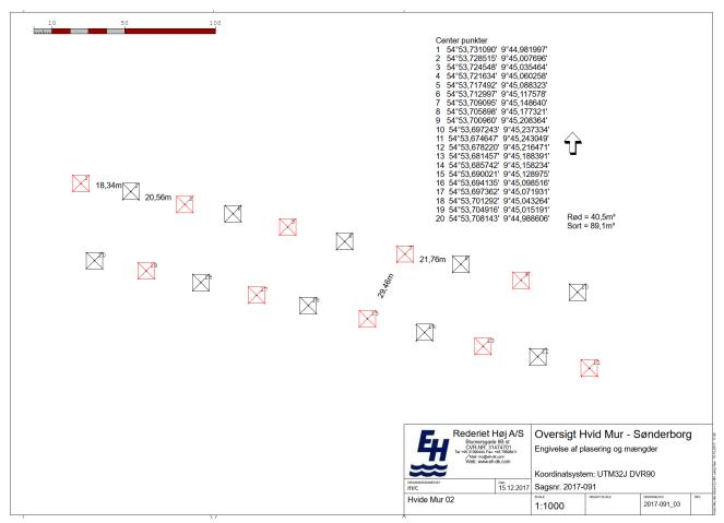
Figure 1.7. Planned reef units at Hvide Mur. Red squares are low reef units, and black squares are high reef units.
