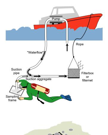
Figure 3.2. Frame sample on a sand cobble covered seabed. Area covered is 1/6 m2 and sampling depth is at least 13 cm into the sediment if possible.
