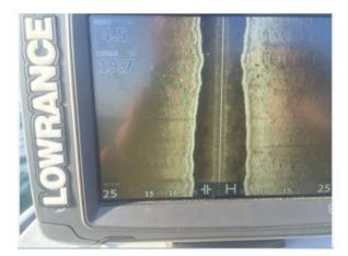
Figure 1.3. Screen pictures of the Lowrance Elite 7Ti instrument used for surveying the seabed in Sønderborg Bay. To the left is a contour plot including waypoints. To the right is a scan of the seabed revealing a scatted cobble reef in Sønderborg Bay.
