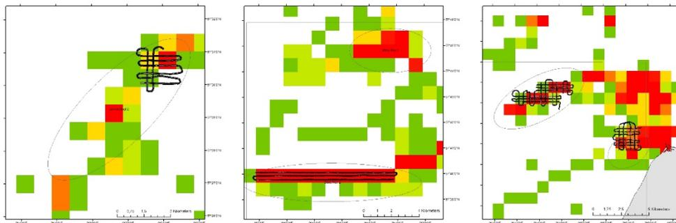
**Figure 4.1.8.** Sail routes for the sidescan survey in Skagerrak. Left panel: Jammerbugt 2 study area, in which four squares were covered, two of these were fully covered and two only in the east-west direction. Middle panel: Store Rev 2 study area, here 10 squares were covered, all only in the east/west direction. Right panel: Hirtshals study area 1 & 2, with seven and four squares covered, respectively.
