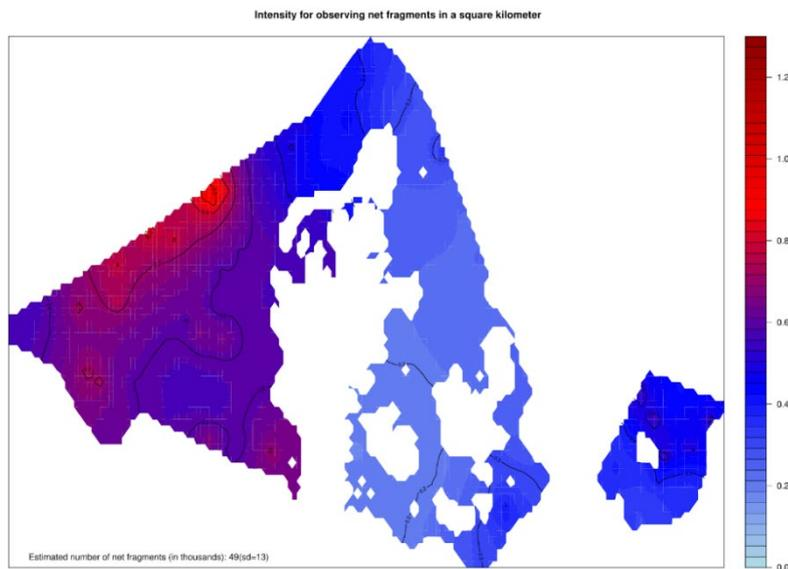
**Figure 5.1.2. (Figure 5.2.9):** The estimated intensity of observing net fragments per square kilometer as estimated from survey data, wreck data and the Swedish dragging survey. The sum over the entire study area (the coloured part of the map) is  $49 \times 10^3$  net fragments with a standard deviation of  $13 \times 10^3$  net fragments.
