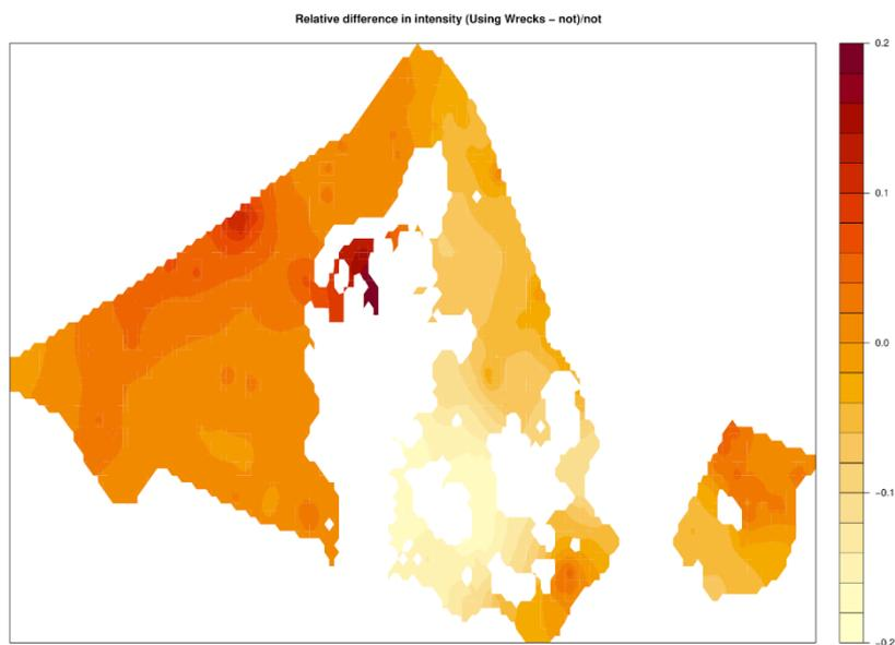
**Figure 5.2.8.** The relative difference in intensity estimates from using the additional observations from shipwrecks.
