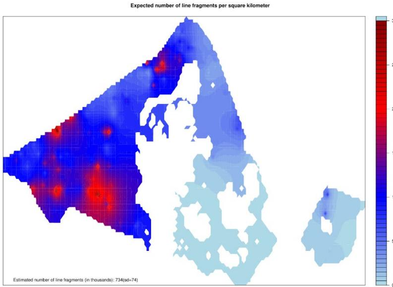
**Figure 5.2.5.** The estimated intensity of observing line segments per square kilometer. The sum over the entire study area (the coloured part of the map) is  $734 \times 10^3$  with a standard deviation of  $74 \times 10^3$ .
