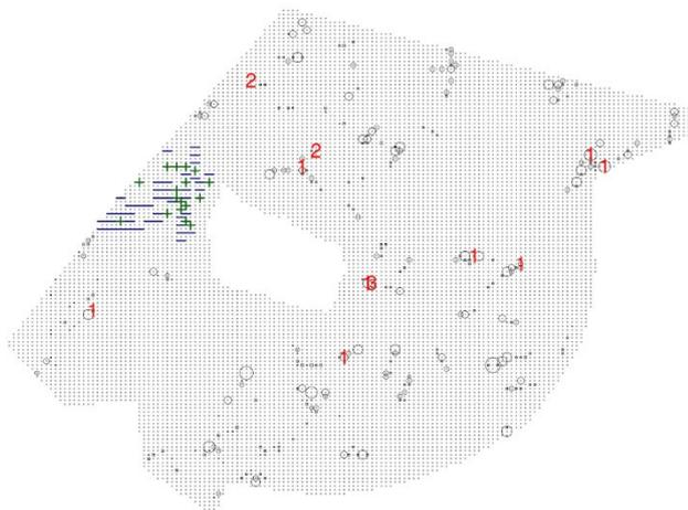
**Figure 5.2.4.** The additional data from the Swedish dragging survey added to part of Figure 5.2.2 (near Bornholm): a blue minus symbol indicates no net fragments found and a green plus symbol indicates that net fragments were found.
