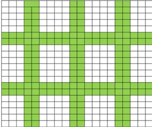
**Figure 4.1.4. Schematic drawing of the survey pattern in a given 1x1 km square. The green areas illustrate the sidescan coverage using a 50 m range on each side.**
