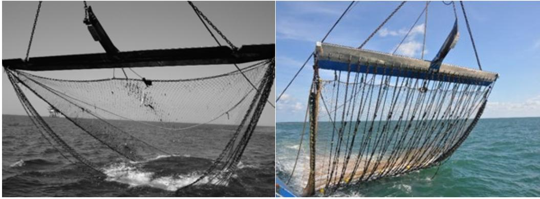
Figure 4.1.1. A conventional Sumwing beam trawl with tickler chains (left) and a Pulse wing with electrodes (right) used in the Dutch beam trawl fishery for sole in the North Sea.
