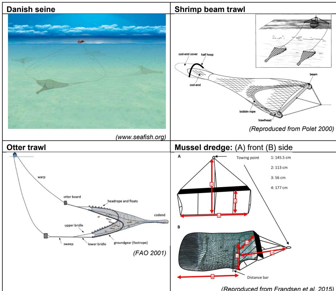
Figure 1.2: Illustrations of the four main bottom towed gears used in Danish coastal areas.
