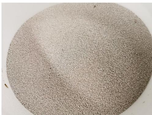
**Figure 53. Struvite material used for enhancing P and N in fish manure cake.**
