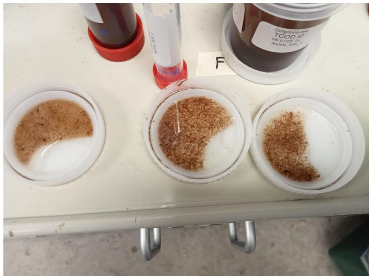
**Figure 27. Physical appearance of coagulated and flocculated sludge.**
