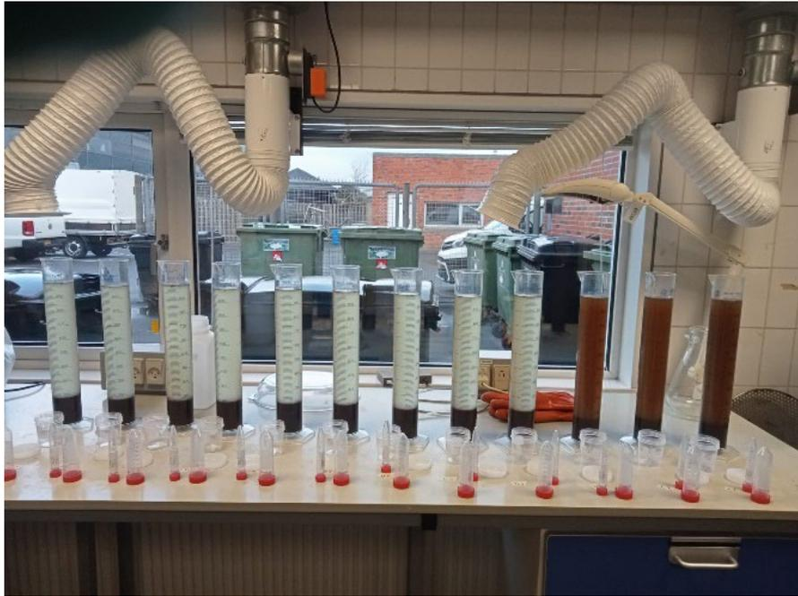
**Figure 26. Coagulation and flocculation jar test screening trials using different chemicals.**
