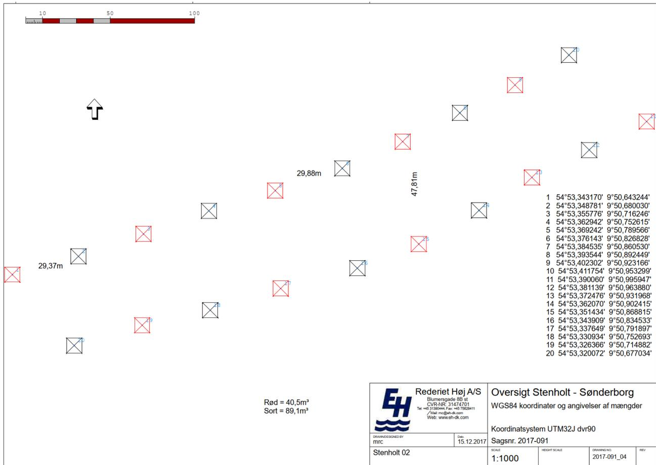
Figure 1.8. Planned reef units at Hvide Mur. Red squares are low reef units, and black squares are high reef units.
