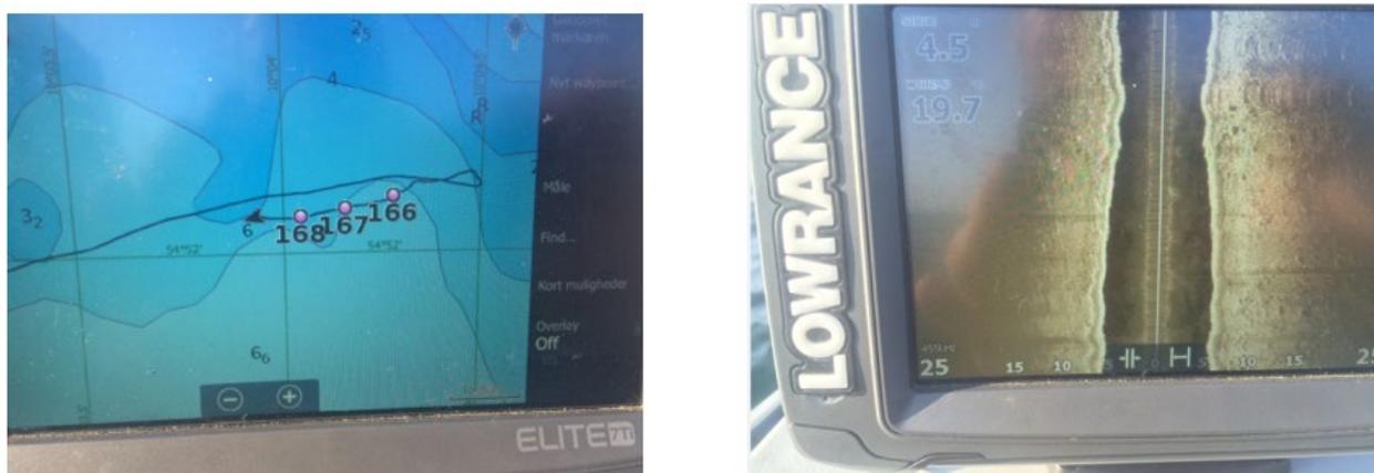
**Figure 1.3. Screen pictures of the Lowrance Elite 7Ti instrument used for surveying the seabed in Sønderborg Bay. To the left is a contour plot including waypoints. To the right is a scan of the seabed revealing a scatted cobble reef in Sønderborg Bay.**
