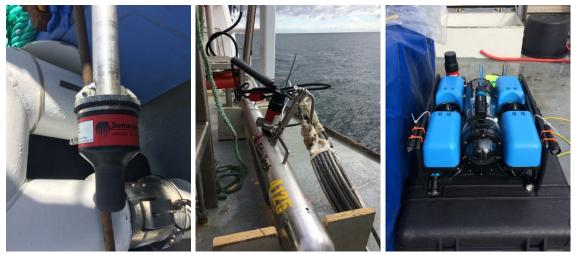
Figure 3. Images of the Sonardyne Micro-Ranger 2, USBL system used on the deployed equipment. Left) The pole-mounted transmitter. Middle) The beacon mounted on the sidescan sonar. Right) The beacon mounted on the BlueRov2. Photo DTU Aqua.
