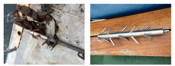
Figure 7. Two types of "x-mass tree" dredges. Left) The dredge used on "Havfisken". Right) The dredge used on "Havørreden", identical to the one used in the Marelitt Baltic project in Sweden.
