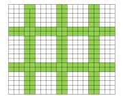
Figure 4. Schematic drawing of the survey pattern in a given 1x1 km square. The green areas illustrate the sidescan coverage using a 50 m range on each side.
