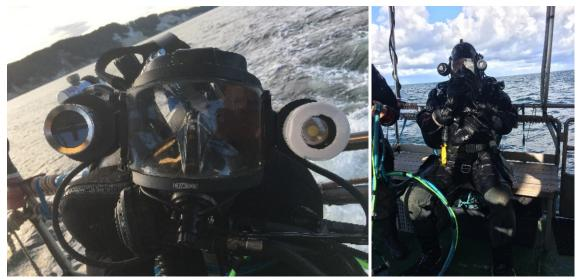
Figure 3. Left) The diving mask mounted with live streaming LH camera and one light. Right) Diver fully dressed and ready to dive
