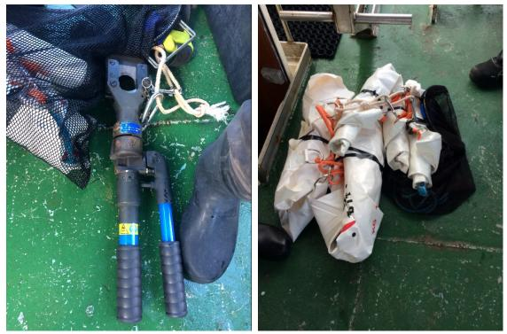
Figure 4. Equipment used for retrieving nets. Left) A wire cutter, Right) rolled up lifting bags.
