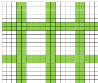
**Figure 4. Schematic drawing of the survey pattern in a given 1x1 km square. The green areas illustrate the sidescan coverage using a 50 m range on each side.**
