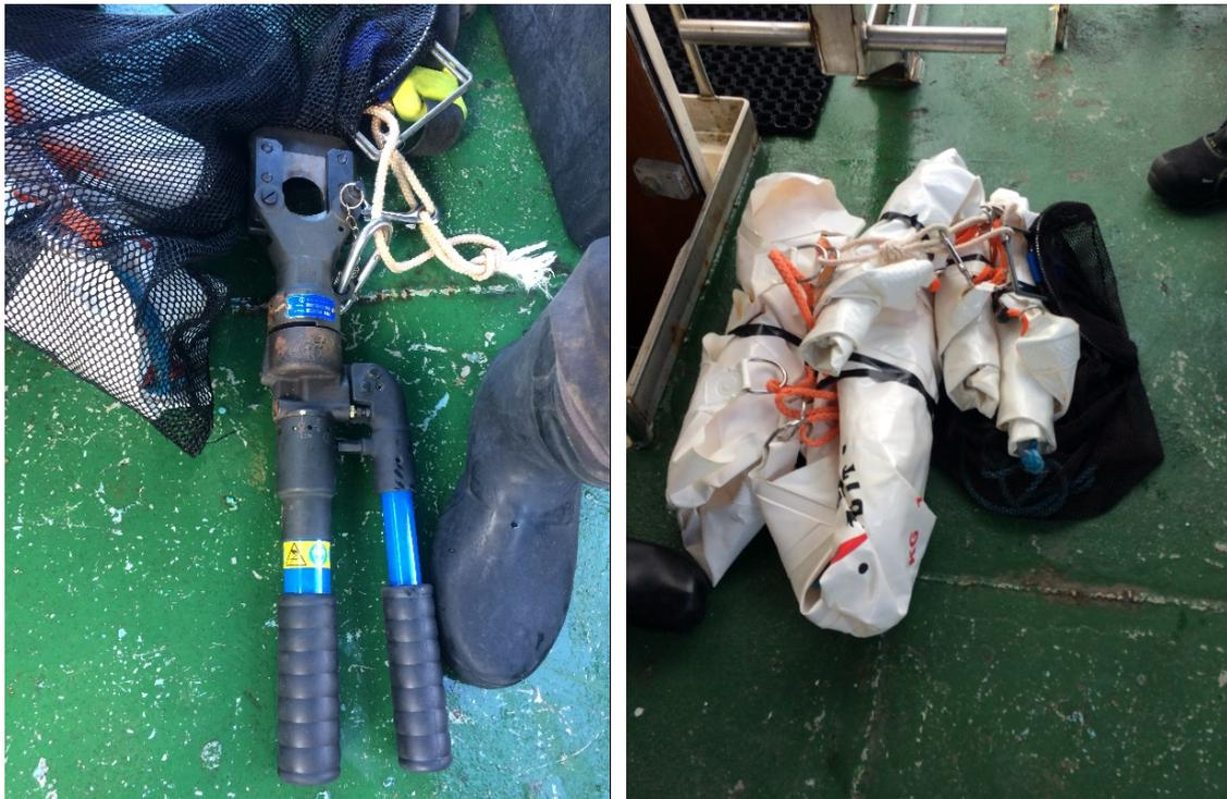
**Figure 4. Equipment used for retrieving nets. Left) A wire cutter, Right) rolled up lifting bags.**
