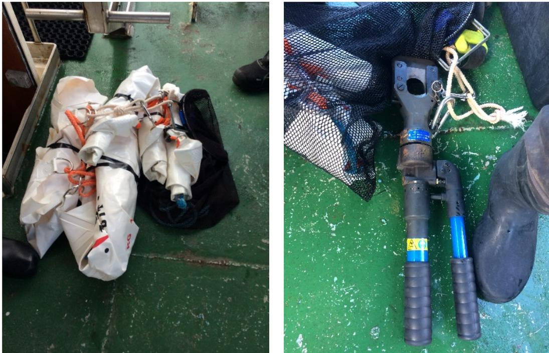
Figure 1. Left) A selection of different sizes of rolled up lifting bags. Right) A hydraulic cable/wire/rope cutter.
