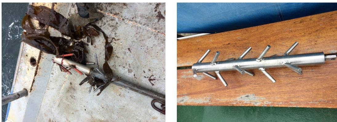
**Figure 7. Two types of ”x-mas tree” dredges. Left) The dredge used on “Havfisken”. Right) The dredge used on “Havørreden”, identical to the one used in the Marelitt Baltic project in Sweden.**
