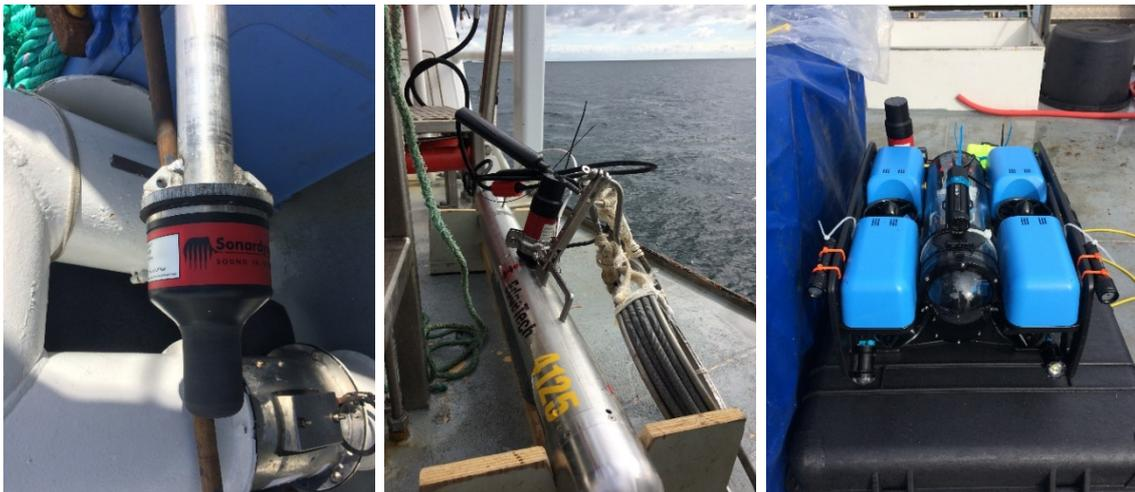
**Figure 3.** Images of the Sonardyne Micro-Ranger 2, USBL system used on the deployed equipment. Left) The pole-mounted transmitter. Middle) The beacon mounted on the sidescan sonar. Right) The beacon mounted on the BlueRov2. Photo DTU Aqua.
