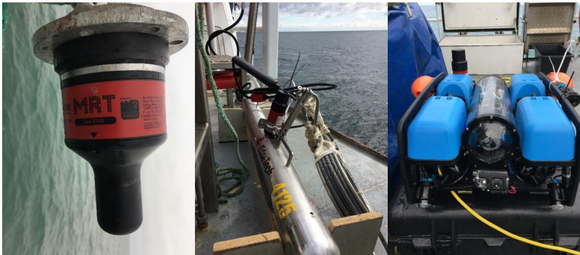
**Figure 3. Images of the Sonardyne Micro-Ranger 2, USBL system used on the deployed equipment. Left panel: The pole-mounted transmitter. Middle panel: The beacon mounted on the sidescan sonar. Right panel: The beacon mounted on the BlueRov2. Photo DTU Aqua.**
