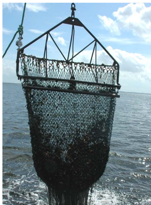
Figur 1. Almindelig muslingeskraber under skylning.
