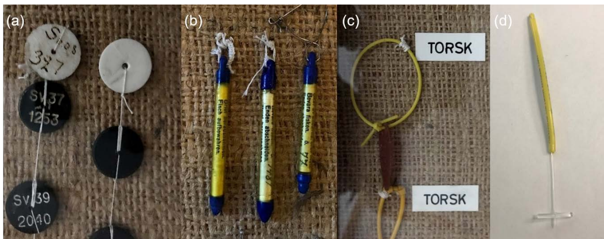
Figure 3. Different types of tag used in the Baltic cod tagging experiments during 1955-1993. Peterson disc tag (a); Lea's hydrostatic tag (b); Carlin tag (c); T-bar (d).
