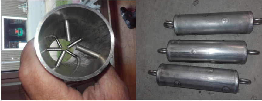
Figure 5.2. Left side: sticks welded to the inside of the pinger. Right side: the three rattle pingers.
