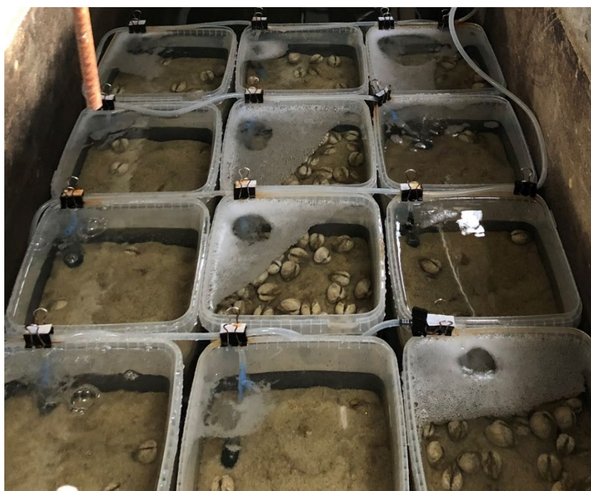
Figure 5.2. Photos of one experimental setup showing containers with cockles and air bubbling. Upon the start of the experiments, surfacing or burial activity was determined by counting the number of surfaced or buried cockles either manually or from images taken with overhanging cameras at variable intervals. Dead cockles were removed when detected and accounted for and were only observed in the distribution experiments (N = 1) and in the oxygen experiment (N = 28). Photo P. Freitas.
