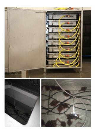
Figure 23. Survival unit to hold fish onboard the vessel (top) and transportation tank to the holding facility with oxygen supply (left and right). Fish were stored in custom-made survival units to minimize the effects of handling, holding and transportation on mortality (Figure 23). The survival units were continuously supplied with running seawater whilst oxygen and temperature were monitored.
