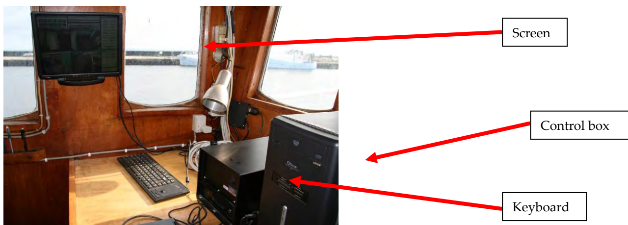
Figure 2. An EM control box in a vessel's wheelhouse.
