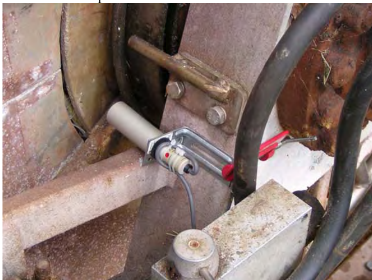
Figure 7 An installed photoelectric drum rotation sensor that tracked vessel setting and hauling events in the sensor data, and functioned as a secondary trigger for video recording.
