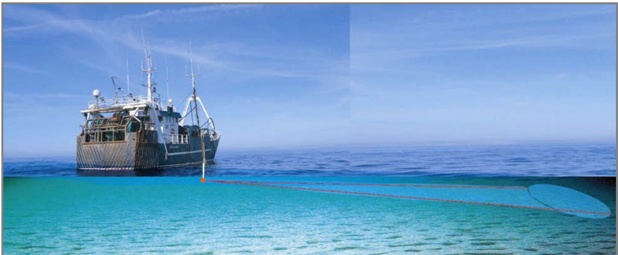
Schematic illustration of horizontal echo beam.
