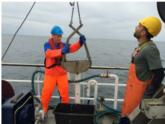
Figure 2.6. The Van Veen grab (seabed area: 0.1m 2 ) deployed in this project to sample sediment and macrobenthos.
