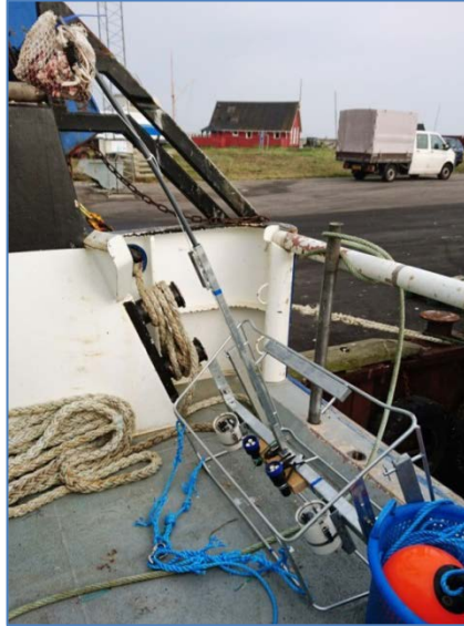
Figure 5.1. Top: SeaGis Stereo BRUV turned 120 degrees counter clockwise on the afterdeck of R/V Havfisken before the research survey. Note the two white camera housings, the two black lamps between the camera houses, and the weights attached to the steel frame. A bait bag made of white netting (in the upper left hand corner of the photograph), and filled with pieces of herring, is mounted on the pole in front of the cameras. During the survey the dark grey plastic pole was removed and the bait bag was fastened to the tip of the stainless rod extending from the frame. This was done to allow visual identification of fish in the turbid waters encountered at some of the deeper stations. The BRUV was left recording on the seabed for one hour after which it was retrieved by means of the blue rope to which a red buoy was attached (seen in the lower right half of the photo). Note that the bait pole and the BRUV both are marked with a single stripe of blue tape, indicating that this is BRUV and pole no. 1. Bottom: The BRUV and pole no. 2 was marked with two stripes.
