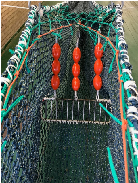
Figure 1. The modified SELTRA codend with floats and grid.
