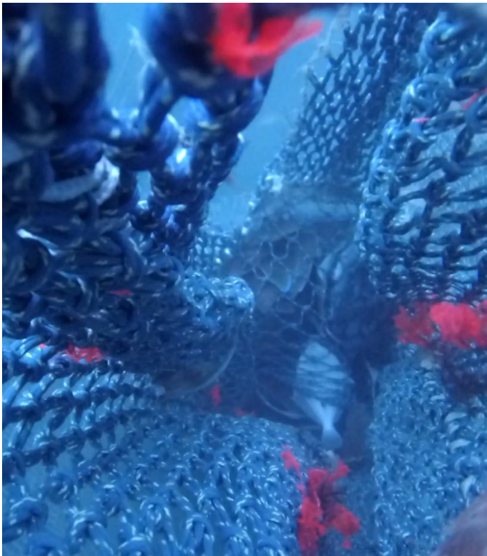
Figure 10. The flip flap net grid acting as a stop net during haul back.
