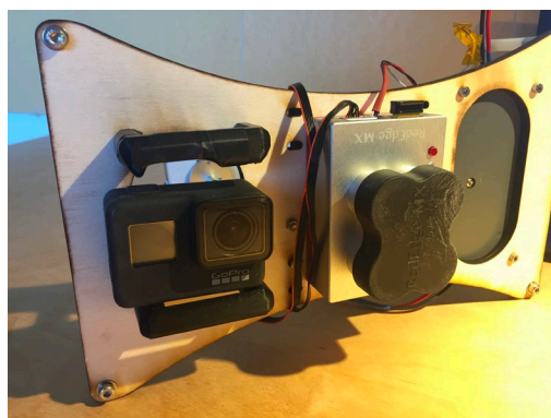
Figure 3.1.1. Setup of the two side-by-side mounted cameras. GoPro camera to the left and the MicaSense RedEdge-MX to the right (Photo: Jonathan Gundorph).
