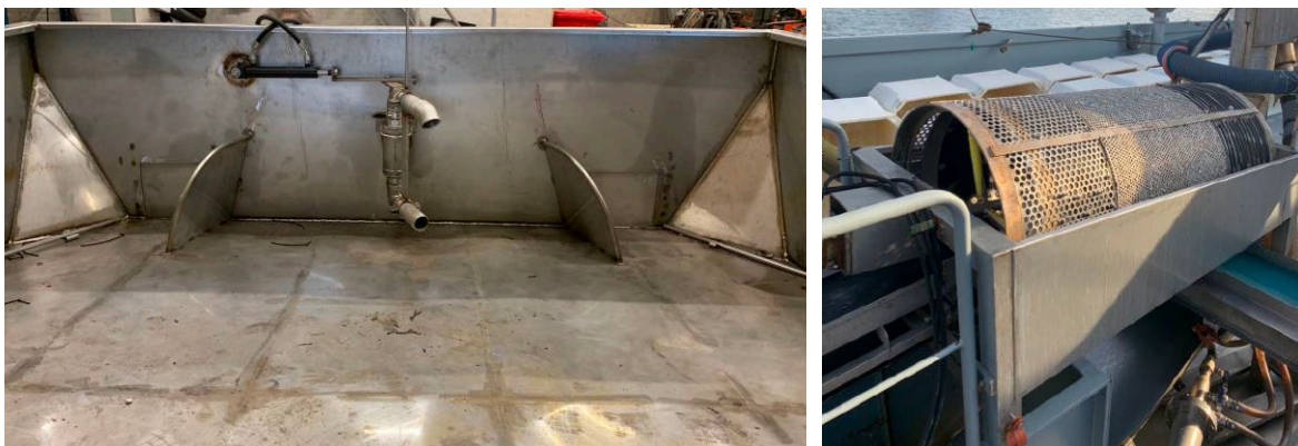
Figure 8.13.1. Left: the inside of one of the sorting tables with the two sliding doors in each corner and the hydraulic washer outlet in the centre. Right: Sorting drum with the conveyor belt at the lower left corner (Photos: Esbjerg Shipyard).
