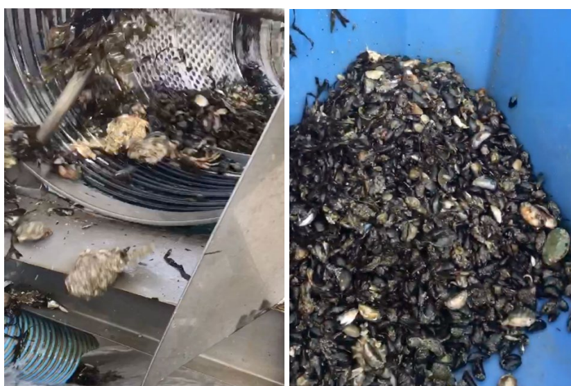
Figure 8.13.4. Left: Sorting drum showing that the separation of the blue mussels occurs at the start of the drum and Pacific oysters and other larger parts are transported to the end of the drum. Right: Sorted clean fraction of blue mussels (Photo: Fiskeriselskabet Cardium A/S).
