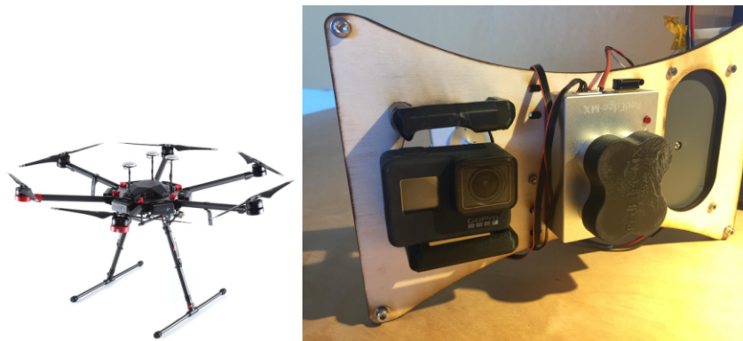
Figure 8: Left: M-600 drone, right: Payload setup: GoPro camera (left camera) and MicaSense RedEdge-MX (right camera)
