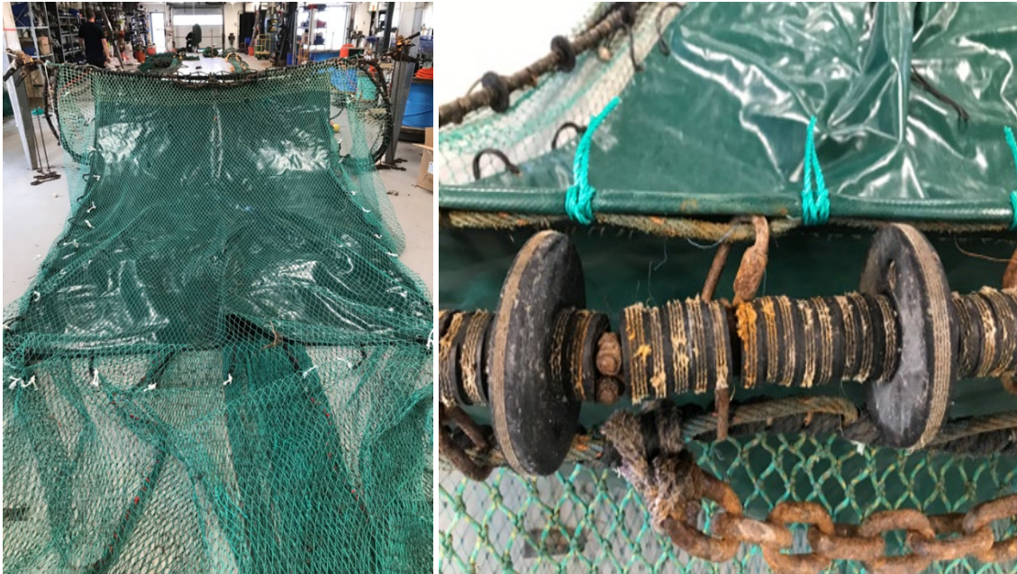
Figure 9. Sediment suppressing sheet installed in the centre of the ground-gear in the Nephrops directed mixed species trawl (FN462 JEANNE). The left picture shows the sediment sheet installed in the lower panel of the trawl, and the right picture shows its attachment forward to the ground gear. The sheet needs to be attached as close to the ground gear as possible.
