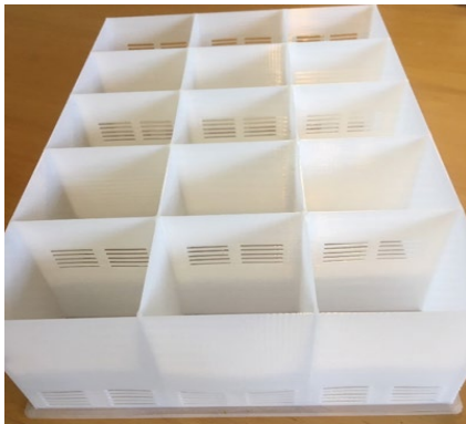
Figure 15. 3D printed unit with 15 chambers and perforated inlet and outlet for water flow.
