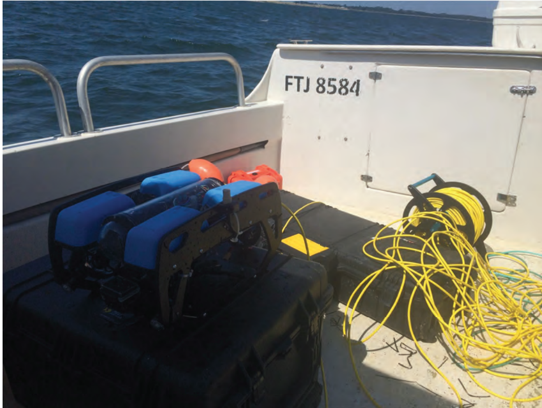
Figure 3.4. The ROV Blue2 with downward facing GoPro attached to battery compartment aboard R/V Fjordrejen.
