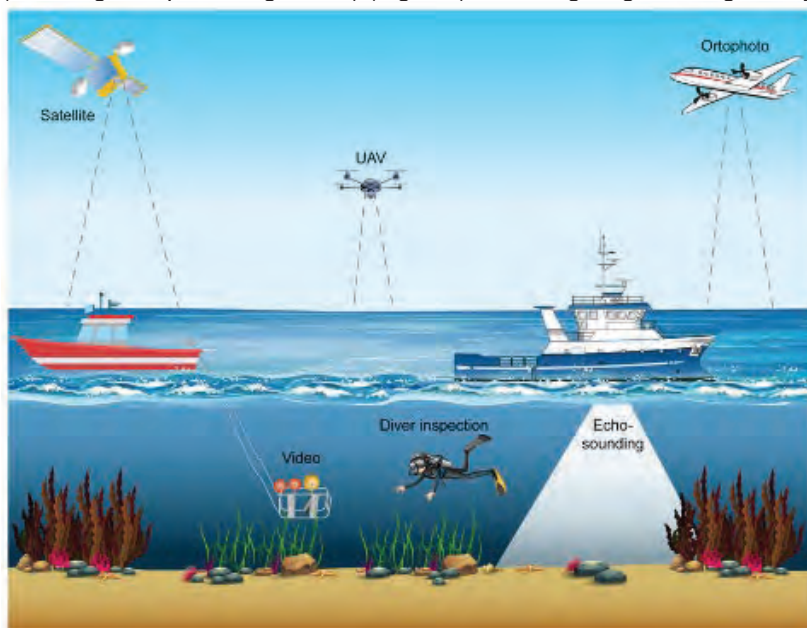
Figure 1.1. Most common monitoring techniques used to map and monitoring seagrasses. From Lønberg et al. 2022.
