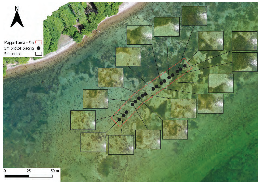
Figure 2.24. Base-map (100 m) with indication of recording of low-altitude (5 m) images based on imagery collected South of Fænø.
