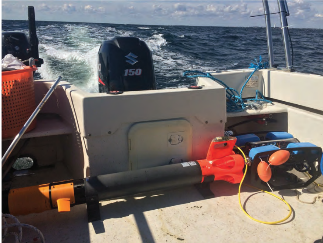
Figure 3.2. The Seagull AUV and Blue2 ROV aboard R/V Havørreden.
