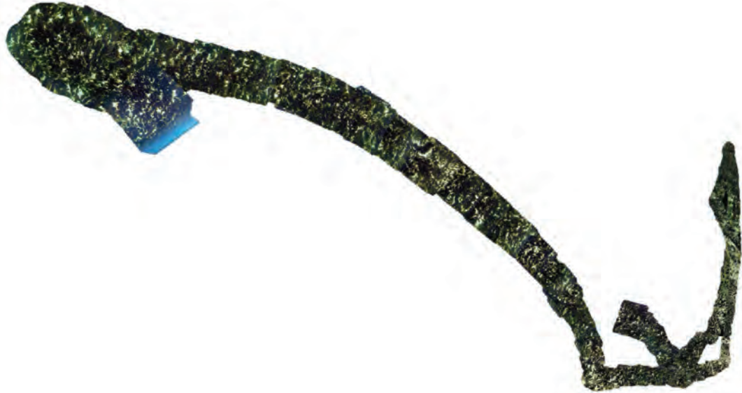
Figure 3.9. An example mosaic produced by the software on the downward facing GoPro. The software uses no external information, besides an initial camera orientation to align the image with north.
